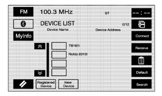
My Info (Information): Select this screen button to display the details of your Bluetooth® device including the name and passkey information. Selecting Device Name allows you to edit the name of the Bluetooth® device name. Selecting PASS-Key® allows you to edit the pairing passkey used for your vehicle. The system default device name is "Cadillac STS" and the PASS-Key® is set to "1234".
